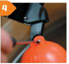
Using a Phillips head screwdriver adjust the float to one of the three positions on the lever to achieve desired water level
