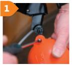
Unscrew the float using Phillips head screwdriver
