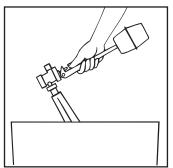
1. Turn off water supply to toilet cistern. Disconnect pipe work and remove old valve from toilet cistern.
