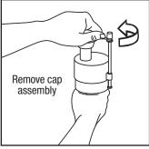
5. Make sure water supply is off. With **RIGHT HAND** push float cup up. (See drawing) Hold valve shaft tight. With **LEFT HAND** grab top cap and
