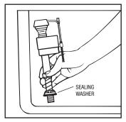
2. Place sealing washer on threaded shank and position valve in cistern, passing threaded shank through hole in cistern.
