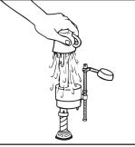
6. While holding a container over the uncapped VALVE to prevent splashing, turn water supply on and off a few times. Leave water supply off.
