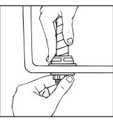
4. Position valve inside cistern and push down on the valve shank. Thread the locknut. HAND TIGHTEN ONLY. DO NOT OVERTIGHTEN OR CISTERN MAY CRACK. Reconnect water supply to valve. Hand tighten nut. HAND TIGHTEN ONLY. DO NOT OVERTIGHTEN OR CISTERN MAY CRACK. Make sure float moves up and down freely. IMPORTANT: See over for supply tube installation.
