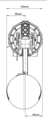
**Standard Float Valve** Side ViewDimensions <sup>3</sup>/<sub>4</sub>" Adaptor
