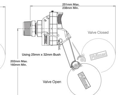
**Standard Float Valve** Side View Dimensions 1-1/4" Adaptor
