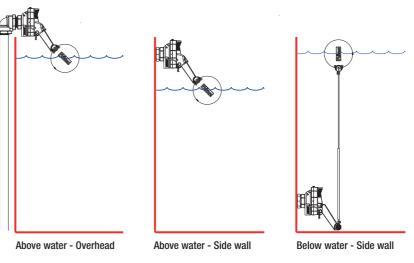
\* Water outlet position can be adjusted by removing the cap and rotating the body 90°
