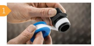
Apply PTFE tape or approved sealant to the male thread. Sufficient tape needs to be applied to ensure a watertight seal.
