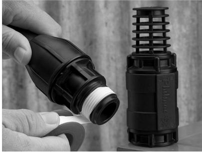
**1.** Apply PTFE tape or approved sealant to the male thread the non-return/foot valve is to be screwed into. Sufficient tape needs to be applied to ensure a watertight seal.
